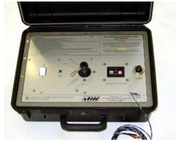
DPD Thruster Bench Test Power Supply is included with DPD Long Term Maintenance Special Tools.
